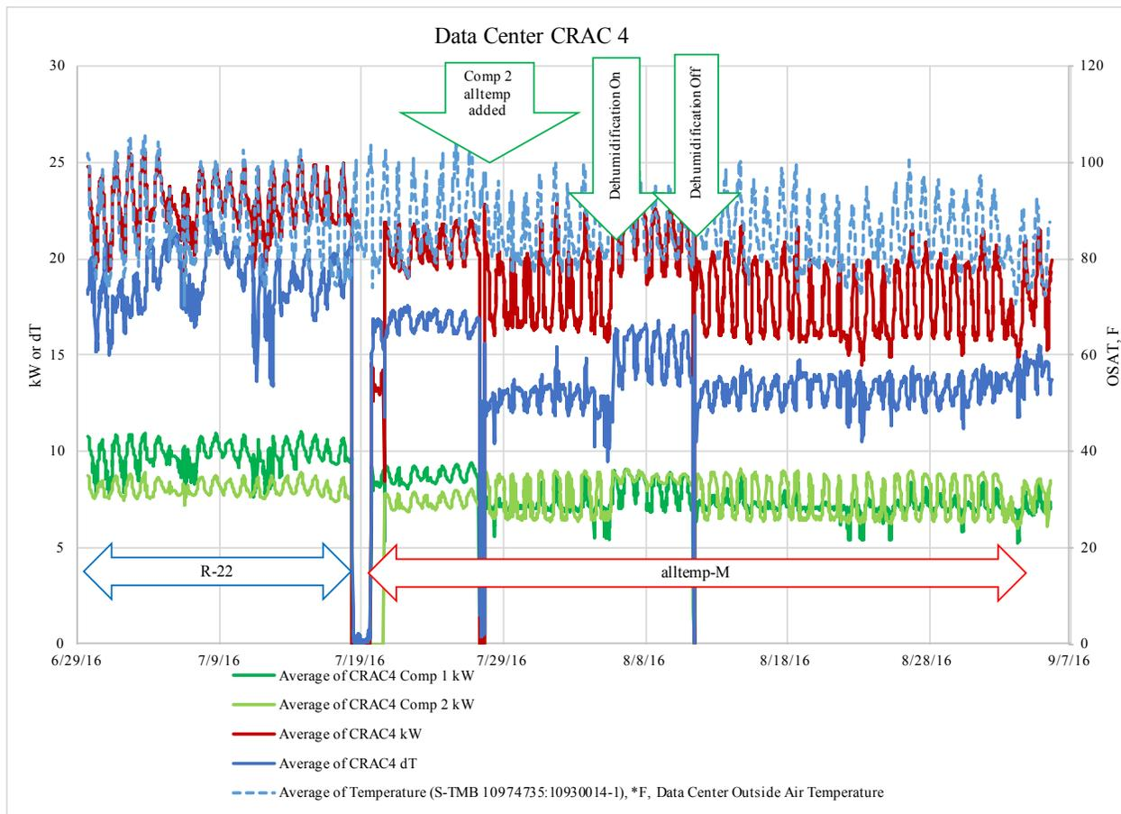
The temperature difference ( $\Delta T$ ) between the return and supply air load is shown as a heavy blue line. Because the CRAC units operate with constant fan speed and therefore constant flow,  $\Delta T$  serves as a proxy for cooling load. Cooling load does appear to decrease with alltemp® operation. Despite the apparent reduction in  $\Delta T$ , CRAC 4 appears to do a better job of maintaining space temperature setpoint than with R-22.
